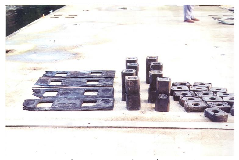
A worn-out set of connector hardware for the original sections of A Dock. These are the buffer pads between the sections on the left, the sheer connectors in the centre, and the bolt bumpers on the right. They have been lasting approximately 15 years and were replaced by a work party in less than a day.
