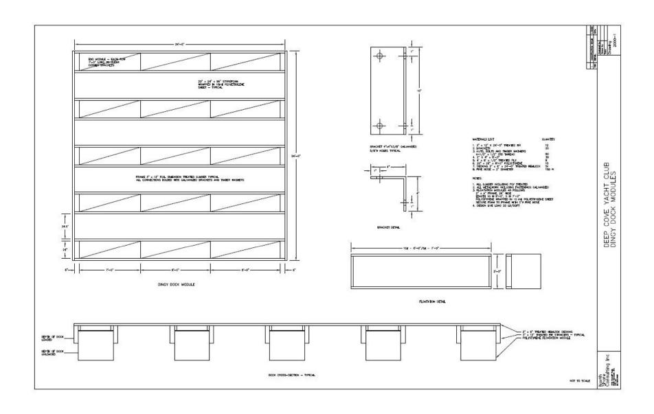
Construction details for a Dinghy Dock Module – Three were built.
