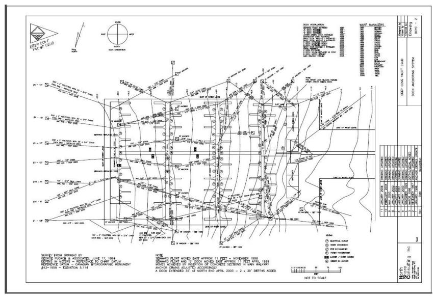
The drawing of the anchoring system pre 2010. The drawing included depths of anchors, inspection dates and other relevant data. Eight additional anchors were added in 2010/2011 to handle the larger boat size.
